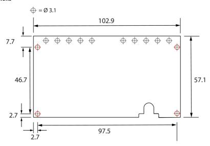
Dimensions in mm; Tolerance acc. to ISO 2768-m
